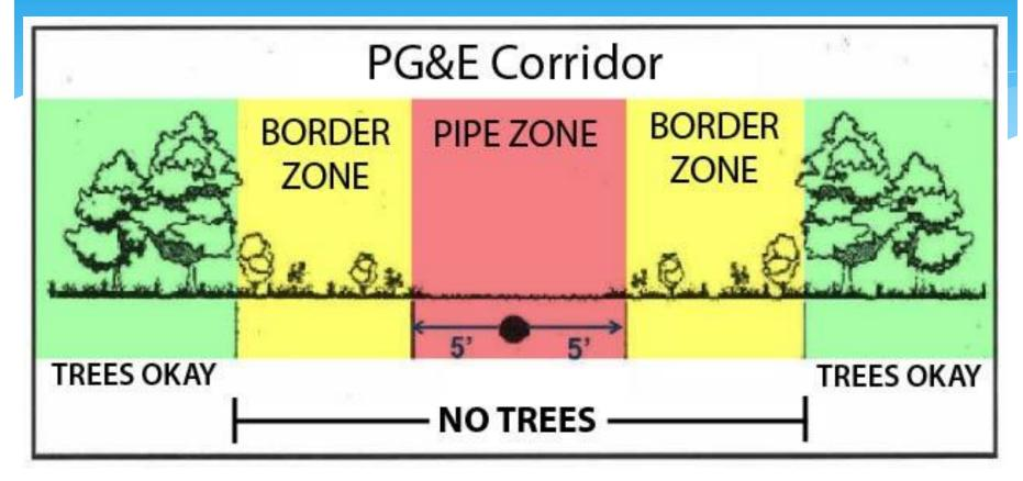
**Pipe Zone-** the Pipe Zone is defined as the area that extends 5 feet from the edge of the pipe on both sides. Planting within this zone restricts vegetation to non-woody, low profile ground covers not to exceed 18 inches in height.
